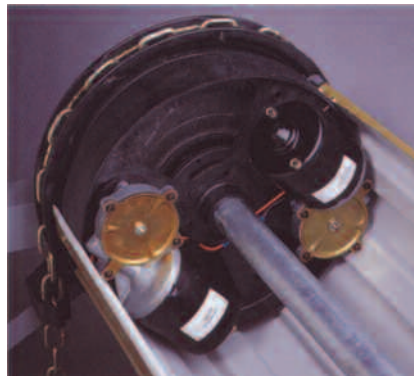
Detail B: Interior view of Dual 1/3 HP DC motors inside the coil of the door. Also shown is the chain hoist sheave, which accepts welded chain and the chain guide.
